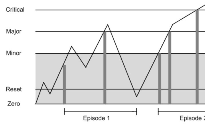
When a counter crosses a threshold for the first time, it triggers a response. A trigger point is represented with a vertical bar in the figure above. The actual response is determined by rules that are described later. For now, let's just say the cache triggers the response rules. Any given threshold (minor, major, or critical) will not trigger a second time for a
